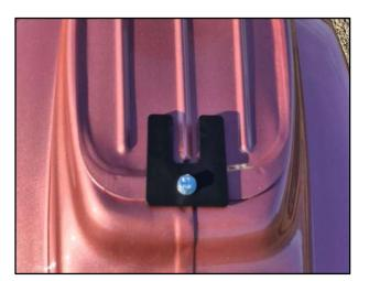
**Step 4:** Fasten the frame plate for the magnet with an M7×20 hex bolt and an M7 washer.
