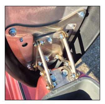
**Step 2:** Pad the hinge with 2 x M7 washers over the threaded holes on the frame to compensate for the height of the frame flange. Then fasten the hinge to the frame using  $2 \times M7x20$  hex bolts and  $2 \times M7$  washers.
