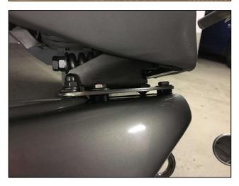
**Step 6:** Fasten the plate to the frame.
