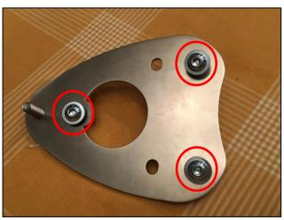
**Step 2:** Insert the three M8x20 lens head bolt with the integrated washer from the opposite site of the plate. Position: see left picture
