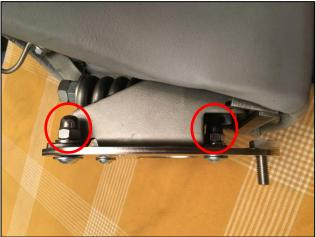
**Step 4:** Fasten the bolts on the plate with the M8 self-locking nuts and M8 washers.
