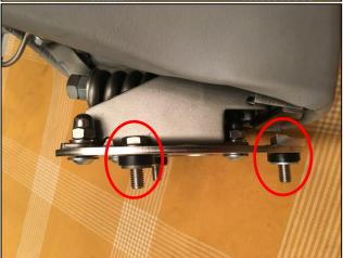
**Step 5:** Insert the remaining two M7x20 hexagon nuts through the holes and put the plastic spacers over the threads.
