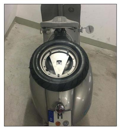
**Step 4:** Place three washers on the bolts and place the spare wheel on the bracket. Fix the wheel to the bracket with three washer and three M8 nuts.
