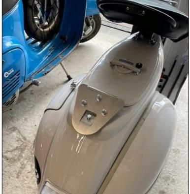
**Step 3:** Mount the spare wheel bracket to the frame of the Vespa with the three M7x20 bolts and washers.
