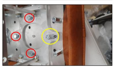
**Step 3:** Install the hinge at the front of the seat with the help of the three M6 self-locking nuts (red circle). Install one M6x20 spacer nut together with a M6 spring ring at the front (yellow circle). Subsequently test if the hinge opens without any problems.
