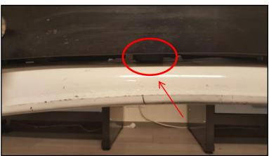
**Step 10:** Screw out the two rubber buffers on the side of the seat until they make contact with the frame. Adjust the rear buffers so they evenly make contact with the frame
