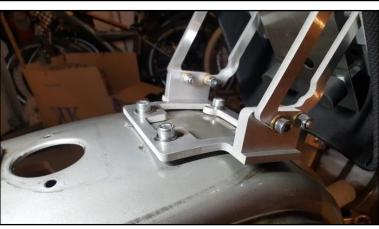
Step 7: Expand the hinge and attach the seat to the front side of the frame by using with the M8x40 allen screws, washers and M8 self-locking nuts (see left picture). Support the hinge on all four holes by placing one or two M8 washers underneath it.
