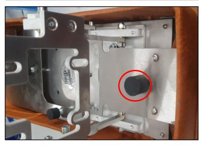
**Step 11:** Look through the front gap between the seat and the frame and screw out the front rubber buffer until it evenly makes contact with the frame. Lock the height by tightening the counter nut underneath the buffer.
