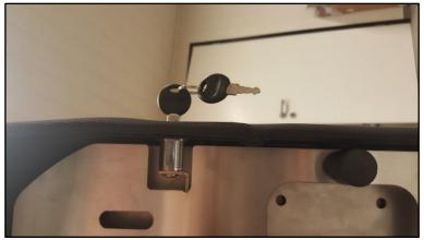
**Step 2:** Change of the lock-orientation. Losen the union nut of the lock cylinder slightly and turn the complete cylinder: Key in horizontal position = unlocked (see left picture)
