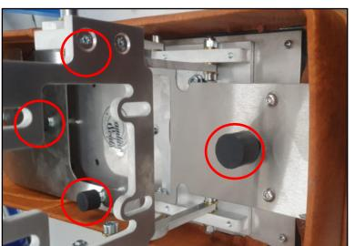
Rubber buffers Front: 1 x D=25 / H=25 Middle and rear: 3 x D=25 / H=15
