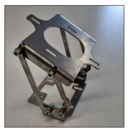
**Step 2:** Mount all four levers at the upper seat-plate with the M6x20 allen bolts, the M6 self-locking nuts and three brass washers.
