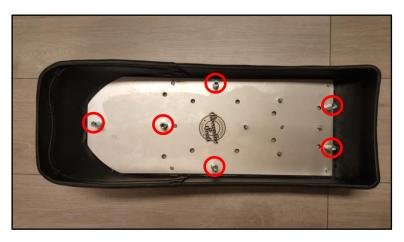
**Step 1:** Mount the 6 x M6 washers, 6 x M6 spring-rings and 6 x M6x20 spacer nuts according to the picture on the left
