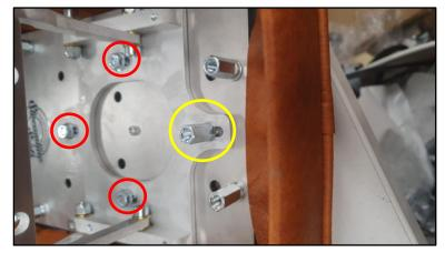
**Step 2:** Install the hinge at the front of the seat with the help of the three M6 self-locking nuts (red circle). Install one M6x20 spacer nut together with a M6 spring ring at the front (yellow circle). Subsequently test if the hinge opens without any problems.
