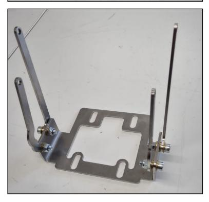
**Step 1:** Mount the short levers at the front and the long levers at the back with the M6x20 allen bolts, the M6 self-locking nuts and three brass washers. Orientation of the levers: See picture on
