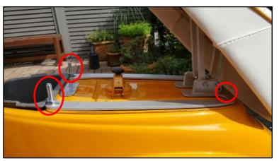
**Step 7:** Attach the seat and the hinge to the frame.
