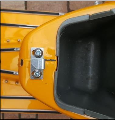
**Step 9:** Attach the new locking bracket to the frame with the M7x20 hexagon bolts and M7 washers. Refer to photo on the left
