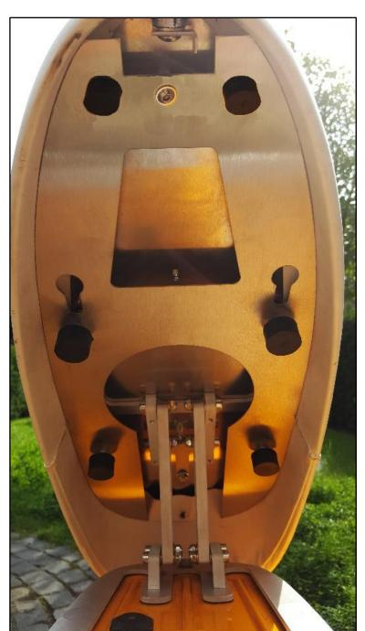
**Step 11:** Adjust the height of the front rubber buffers so they evenly lie on the frame when the seat is closed and the seat can still be locked when slightly pressing on the tip.
