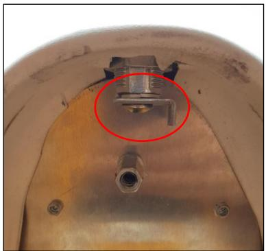
**Step 3:** Remove the original rubber buffers, the screws and the cover plate.
