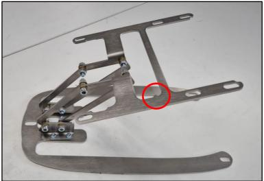
**Step 3:** Attach all four levers to the upper seat-plate with M6x20 allen bolts, the M6 self-locking nuts.
