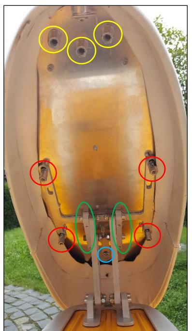
Step 6: Mount the hinge on the lower plate of the seat with the spacer nuts and M6 washers (Red marking). Use the M6 self-locking nut in the back (Blue marking).
