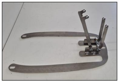
**Step 2:** Attach the short levers at the back and the long levers at the front of the base plate with the M6x20 allen bolts and the M6 self-locking nuts.
