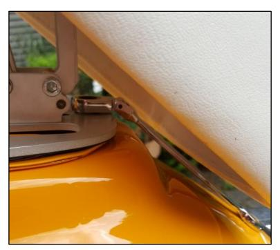
**Step 8:** Tighten the rear screw using the flexible ratchet, if available.
