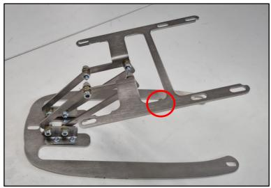
**Step 3:** Attach all four levers to the upper seat-plate with M6x20 allen bolts, the M6 self-locking nuts.
