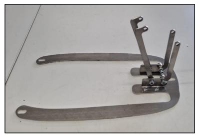
**Step 2:** Attach the short levers at the back and the long levers at the front of the base plate with the M6x20 allen bolts and the M6 self-locking nuts. Place three brass washers between the
