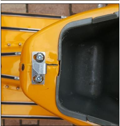
**Step 7:** Attach the locking bracket to the frame with the M7x20 hexagon bolts and M7 washers. Refer to photo on the left. Position the locking bracket completely to the front initially as the final placement will need to be adjusted later.
