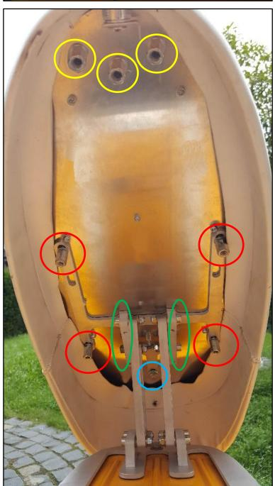
Step 4: Mount the hinge on the lower plate of the seat with the spacer nuts and M6 washers (Red marking). Use the M6 self-locking nut in the back (Blue marking).
