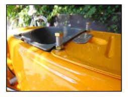
**Step 5:** Screw in the two M7x40 hexagon bolts in the front and the M7x40 slotted-head bolt at the back of the tank together with the M7 washers and nuts.
