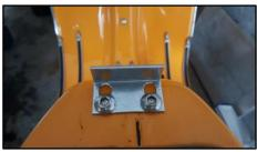
Step 8: Mount the locking bracket to the front of the frame together with the two M7x20 hexagon bolts and M7 washers as shown on the photo to the left. Place the bracket completely to the front and tighten the bolt.
