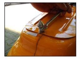
**Step 3:** Remove the cone bolt for the locking mechanism of the old seat.
