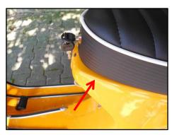
Step 7: Look through the front slit between the seat and the frame and adjust the height of the two front rubber buffers until they sit closely to the frame. Secure the height of the buffers by tightening the counter-nuts.
