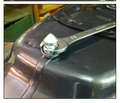
Step 3: Remove the cone bolt for the locking mechanism of the old seat.
