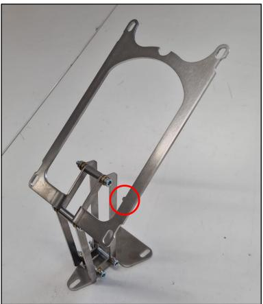
Step 3: Attach all four levers to the upper seat-plate with two M6x55 allen bolts, the M6 self-locking nuts and four brass washers. Place the two metal spacers between the allen bolts and the brass washers between the allen bolts, the levers and the seat-plate. Orientation of the seat-plate: see picture
