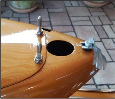
**Step 7:** Screw in the two M7 headless screws together with the M7 nuts and washers appr. 10 mm into the front of the tank.
