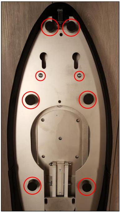
**Step 11:** Mount the cover plate with the two M6x10 lens head bolt, six rubber buffers and six M6 washers.
