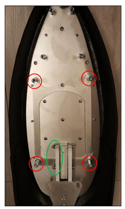
**Step 8:** Attach the seat to the hinge as seen on the left and secure it with the four M6x20 spacer nuts and M6 spring rings.
