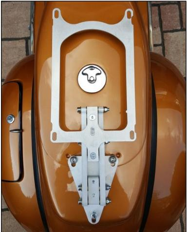
**Step 5:** Attach the hinge on the frame with the three M7x20 hexagon screws and washers.
