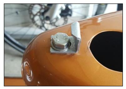
**Step 6:** Attach the locking bracket to the frame with the M7x20 hexagon bolt and M7 washer. Direction: see photo on the left.
