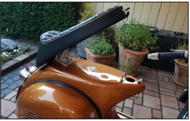
**Step 12:** Unlock the seat by slightly pressing on the front tip. Hold the back of the seat while opening so the composite leather doesn't collide with the frame during the opening process.
