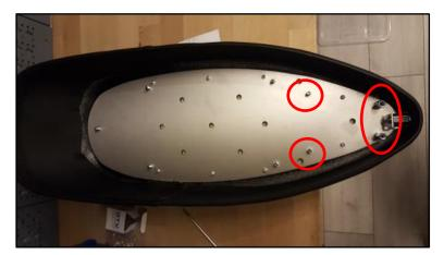
**Step 4:** Screw in the four M6x20 spacer nuts together with the M6 washers and M6 spring rings on the four front riveted threads.
