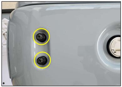
**Step 5:** Insert the two 20 mm diameter spacers into the two front frame recesses and screw tight with the M8x40 screws.
