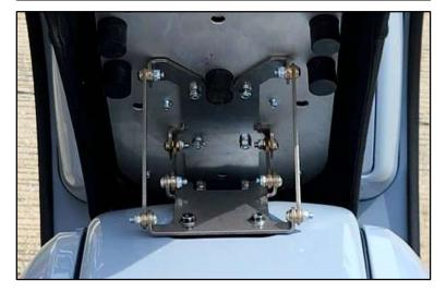
**Step 9:** Screw the seat to the frame using the two M8x40 Allen pan-head screws with flange.
