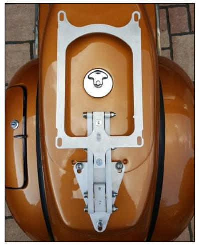
**Step 5:** Attach the hinge to the frame with the three M8x20 allen bolts and M8 washers. If necessary, horizontally level the hinge
