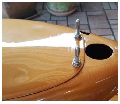
**Step 7:** Screw in the two M8 headless screws together with the M8 nuts and washers appr. 10 mm into the front of the tank.
