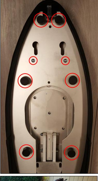
**Step 11:** Mount the cover plate with the two M6x10 lens head bolt, six rubber buffers and six M6 washers.
