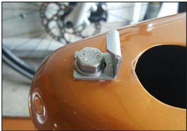
**Step 6:** Attach the locking bracket to the frame with the M8x20 allen bolt and M8 washer. Direction: see photo on the left. Hold the bracket in its position with a plier while fastening the screw.
