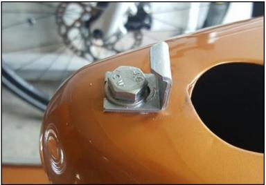
**Step 4:** Attach the new locking bracket to the frame with the M8x20 allen bolt and M8 washer. Refer to photo on the left. Hold the bracket in its position with a plier while fastening the screw.
