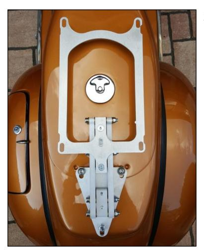
**Step 3:** Attach the hinge to the frame with the three M8x20 allen bolts and washers. If necessary, horizontally level the hinge by using appropriate washers in the back.
