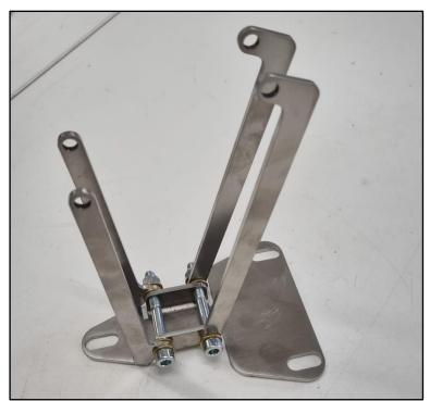
**Step 2:** Attach the long levers at the back of the base-plate with one M6x55 allen bolt, a M6 self-locking nut and four brass washers. Place the brass washers between the allen bolts, the levers and the base-plate.
