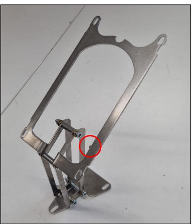
Step 3: Attach all four levers to the upper seat-plate with two M6x55 allen bolts, the M6 self-locking nuts and four brass washers. Place the two metal spacers between the allen bolts and the brass washers between the allen bolts, the levers and the seat-plate.
