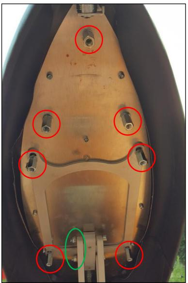
**Step 9:** For seats V2.0: Screw in the three M6x20 spacer nuts together with the washers and retainer rings at the front of the seat
