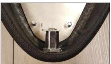
Step 8: Hold the lock cylinder in its position with an appropriate spanner and remove the front screw with a large screwdriver (no cross slot!).
