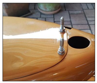
**Step 5:** Screw in the two M8 headless screws together with the washers and nuts appx. 10 mm into the front of the tank.
