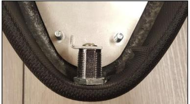
**Step 8:** Hold the lock cylinder in its position with an appropriate spanner and remove the front screw with a large screwdriver (no cross slot!). Replace the old locking shackle with the new one according to the photo on the left.
