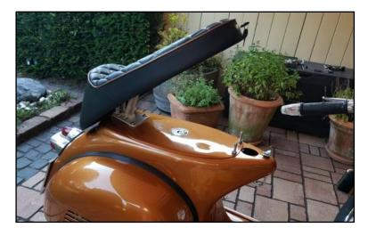
**Step 14:** Unlock the seat by slightly pressing on the front tip. Hold the back of the seat while opening so the composite leather doesn't collide with the frame during the opening process.
