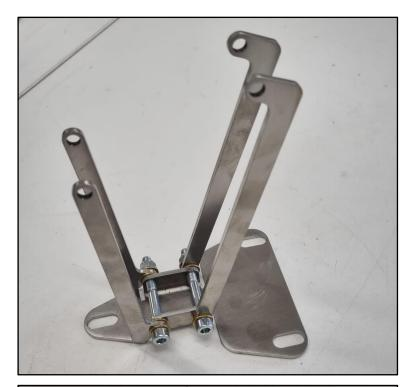
**Step 2:** Attach the long levers at the back of the base-plate with one M6x55 allen bolt, a M6 self-locking nut and four brass washers. Place the brass washers between the allen bolts, the levers and the base-plate. Orientation of the levers: See picture on the left
