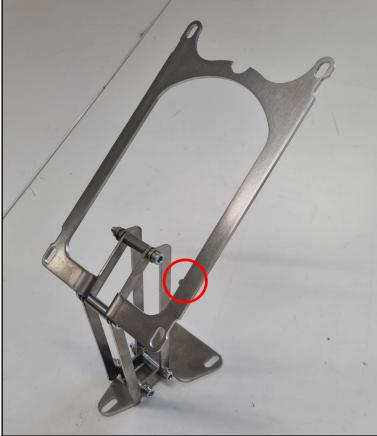
**Step 3:** Attach all four levers to the upper seat-plate with two M6x55 allen bolts, the M6 self-locking nuts and four brass washers. Place the two metal spacers between the allen bolts and the brass washers between the allen bolts, the levers and the seat-plate. Orientation of the seat-plate: see picture on the left. The notch must be on the right side.
