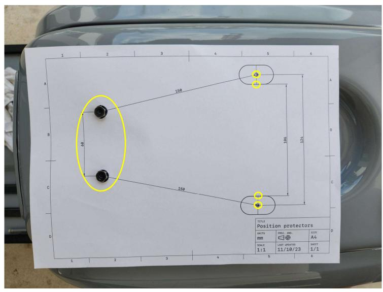
Remove the two front circles from the template and create four small holes in the paper where the protectors will be positioned. Align the template over the two front screws..
