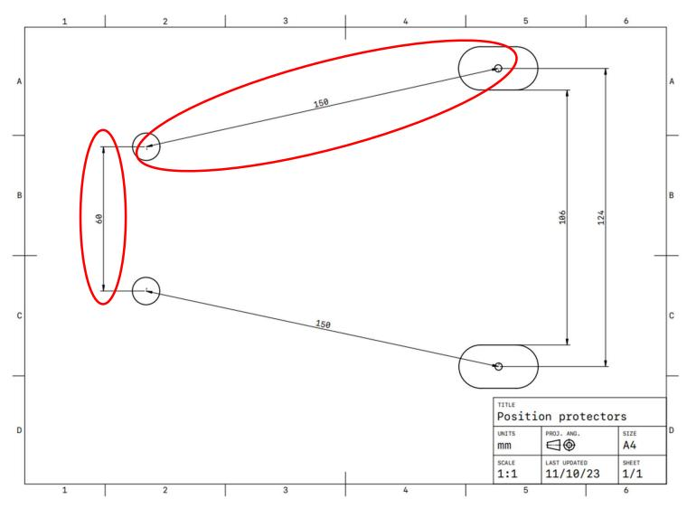
Generate a hard copy of the template at a 1:1 scale, then use a ruler to verify the accuracy of the indicated distances above
