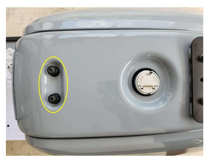
Fasten the two bolts along with the spacers at the front of the frame.
