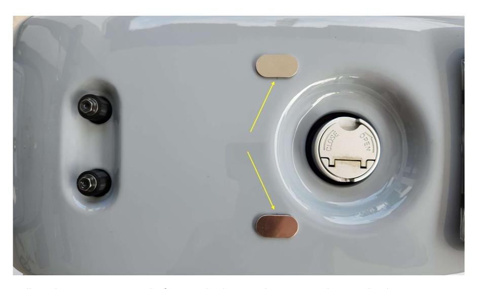
Adhere the two protectors to the frame at the designated positions as shown in the above picture.
