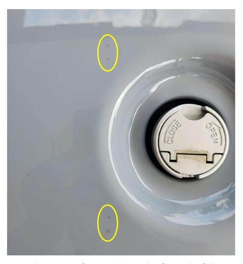
Use a pencil to create four marks on the frame by following the template.
